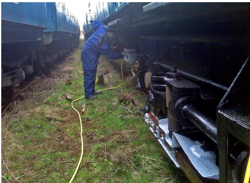
Darren Franklin works on the underframe of DMSB 61727. The grey in the foreground is the refurbished shoebeam. A Mutton.
