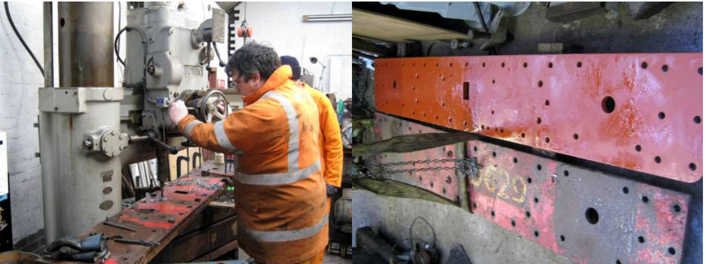
Above Left—Mark Vrettos carefully drills one of the buffer beams and above right old and new beams side by side. Both Peter Drummond
